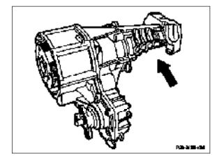
For models with automatic transmission: transfer case with short rear cover (arrow).
