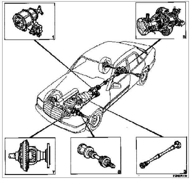
Transfer case Front-wheel drive propeller shaft Rear axle differential (ASD)
